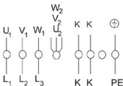
3~ motor, 2 speeds (D/Y switch over) with temperature sensor.
